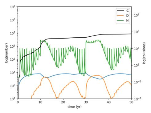
The second is a test of a Starlink style NCell system. For the full model, 3 different types of satellites are used. Each was launched at a rate of 1000 per year to 600, 750, and 900km bands respectively. The result was surprisingly stable for a bit, as seen in the plot of live satellites
