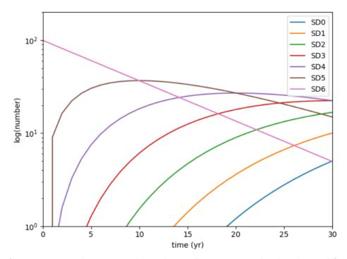
Again, very similar, just without the oscillations since the de-orbiting lifetimes were constant with time and uniform across the system. In the full model, we were also able to run a test of the satellites ascending through the cells. This was run with a launch rate of 50 per year and an ascension lifetime of 0.5yr for each cell, giving the following result
