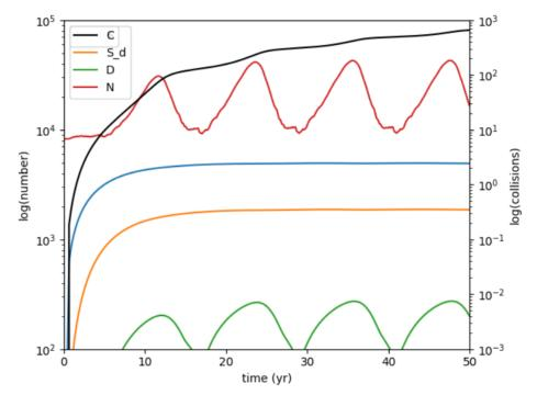
where the blue line is the total number of live satellites in the system. The number of derelicts and debris show periodic patterns of growth and decay, which follow the changes in decay lifetimes due to the solar cycle. The noascending model predicts identical results in this case, since there's no layers of atmosphere in the model to ascend through. For the model removing deorbits, the results are essentially the same
