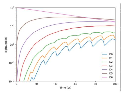
albeit with smaller decay lifetimes, as the derelict satellites have a higher area-to-mass ratio. Rocket body decays were tested as well, with the same area-to-mass ratio as the satellites, and unsurprisingly gave an identical result to the derelict satellites. In the full and no-ascending models, the deorbiting of satellites from the top to bottom cell with a de-orbiting lifetime of 10yr, was also tested, giving the following result
