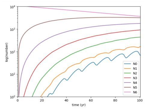
We can see the debris flow downwards as expected. The effects of the solar cycle are much more pronounced in lower cells, likely because of the smaller decay lifetime scales of those altitudes. A similar result is seen in the derelict flow test
