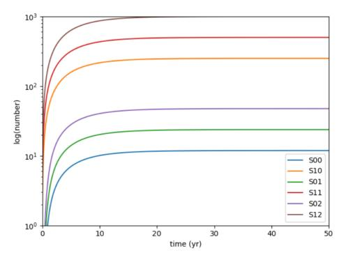
and the same for the minimal model, but monitoring the number of derelict satellites in the shell below
