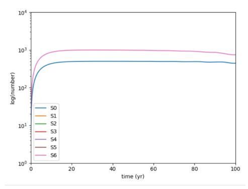
the equilibrium values are as expected, but the cause of the slight downtick near the end of the simulation is not currently known, but is likely from a buildup of derelict satellites in the shells over time, as live satellites fail to go into de-orbit properly. However, if this was the case we'd expect to see the same effect in the minimal model, and this is not what we found
