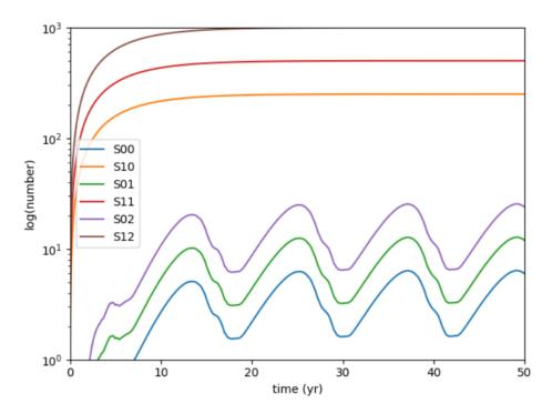
Finally, there's two larger tests that were run in all models. The first is a discrete event test, which is based on the original Starlink test. For the full model, the added events are a custom event which injects  $10^6$  pieces of low-area-to-mass debris at 10 and 30 years, and 10 standard rocket body explosion events per year. The result is as follows, and the discrete events can be clearly seen.
