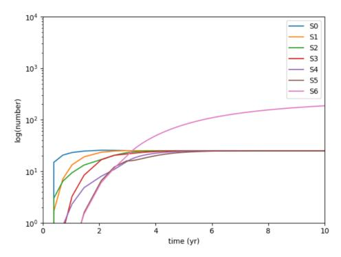
We can see the satellites moving up through the system in the first 5 years or so before things reach an equilibrium, and the top cell eventually (although later than shown in this plot) reaches an equilibrium of 250 satellites, exactly what we'd expect given that the satellite lifetime is 5yr. For the no ascending model, we instead launch all the satellites into the top and bottom shell
