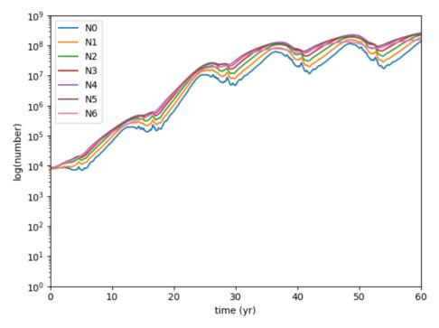
For the no-ascending model, the launch rates are adjusted. The 600km satellites still have a launch rate of 1000 per year, 750km is 500 per year, and 900km is 100 per year. The result is a more stable system, as seen in the plot of live satellites
